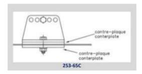
The minimum area of contact between bodyshell /chassis and counter plate is 40cm<sup>2</sup> for each fixing point.
